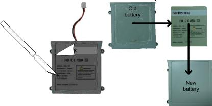
9. Install the new battery using the reverse procedure of the removal of the old battery.
